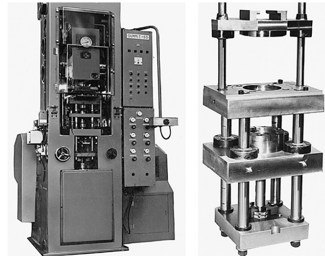
Figure 18-3 (Left) Typical press for the compacting of metal powders. A removable die set (right) allows the machine to be producing parts with one die set while another is being fitted to produce a second product. (Courtesy of Alfa Laval, Inc., Warminster, PA.)
