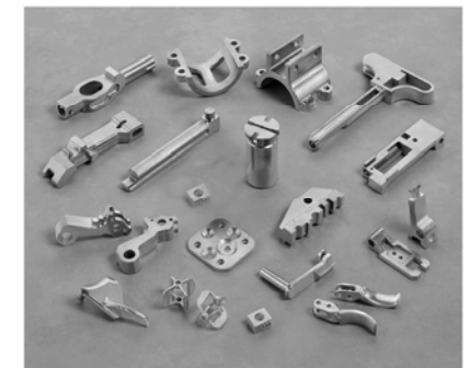
Figure 18-13 Metal injection molding (MIM) is ideal for producing small, complex parts. (Courtesy of Megamet Solid Metals, Inc., St. Louis, MO.)
