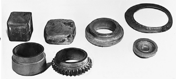
Figure 18-14 (Right) Comparison of conventional forging and the forging of a powder metallurgy preform to produce a gear blank (or gear). Moving left to right, the top sequence shows the sheared stock, upset section, forged blank, and exterior and interior scrap associated with conventional forging. The finished gear is generally machined from the blank with additional generation of scrap. The bottom pieces are the powder metallurgy preform and forged gear produced entirely without scrap by P/M forging. (Courtesy of GKN Sinter Metals, Auburn Hills, MI.)
