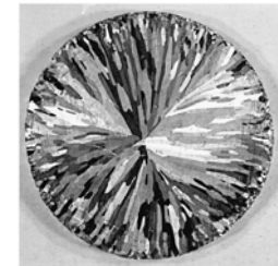
Cross section of a 4-in.-diameter case copper bar polished and etched to show the as-cast grain structure.
