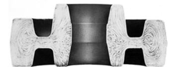
Flow structure of a hot-forged gear blank. Note how flow is parallel to all critical surfaces. (Courtesy of Bethlehem Steel Corporation, Bethlehem, PA.)
