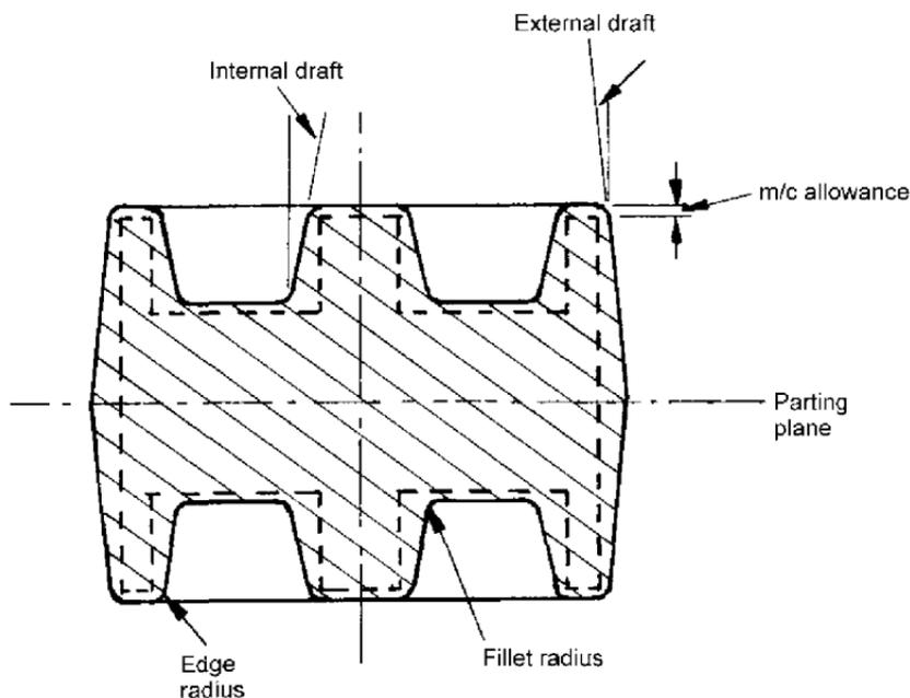
FIG. 14.6 Forging allowances for finish machining and draft.
