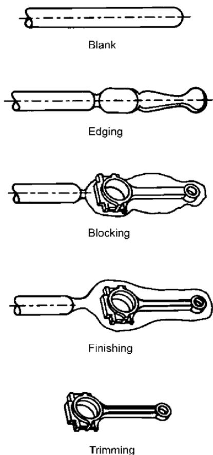
**FIG. 14.8** Typical forging sequence for a connecting rod. (From Ref. 1.)
