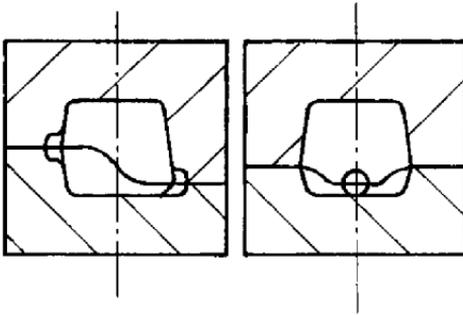
**FIG. 14.1** Forging requiring a cranked parting line.
