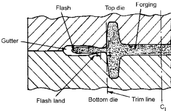
FIG. 14.3 Flash land and flash gutter configuration.
