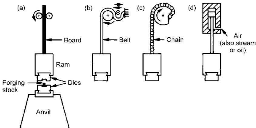
**FIG. 14.17** Schematic of various types of drop hammer. (a) Board hammer. (b) Belt hammer. (c) Chain hammer. (d) Airlift hammer. (From Ref. 1.)
