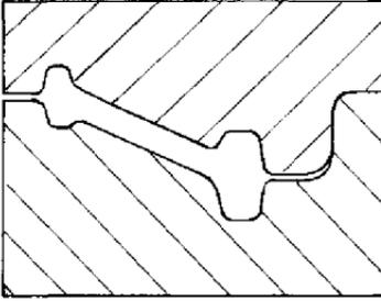
**FIG. 14.13** Typical die lock configuration. (From Ref. 2.)
