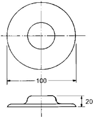
**FIG. 14.4** Steel forging for sample calculations.
