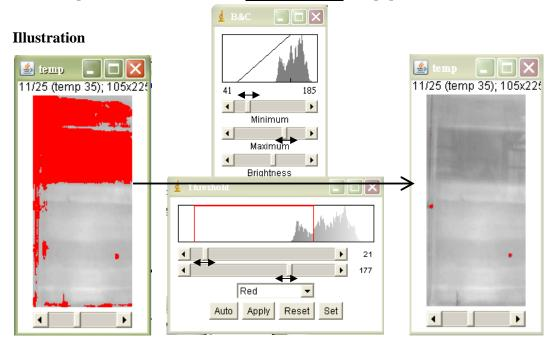
7. Track the particles: after you are satisfied with the binary images of falling spheres, go to Plugins→Stacks→
