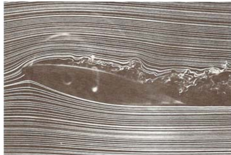
Figure 28 Smoke-wire visualization for a smooth NACA 66,-018 airfoil at an angle of attack of 12^\circ and chord Reynolds number of 40,000. (Courtesy of T. J. Mueller and S. M. Barill, University of Notre Dame.)
