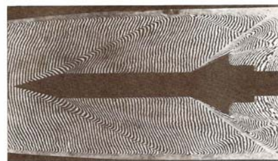
Figure 24 Flow over sharp-tipped spike with conical flare; pressure 100 psia; Ma = 2.98 . (Continued) (c) Wedge-fringe interferogram. [From [40].]
