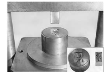
Figure 16-56 Hubbing a die block in a hydraulic press. Inset shows close-up of the hardened hub and the impression in the die block. The die block is contained in a reinforcing ring. The upper surface of the die block is then machined flat to remove the bulged metal.
