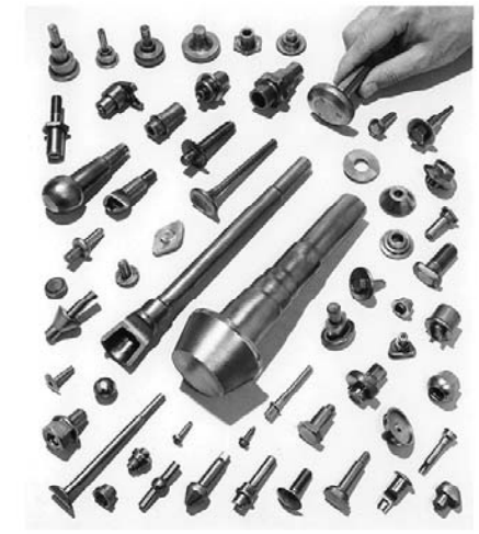
Figure 16-47 Typical parts made by upsetting and related operations. (Courtesy of National Machinery Co., Tiffin, OH.)
