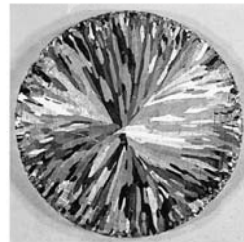
Cross section of a 4-in.-diameter case copper bar polished and etched to show the as-cast grain structure.
