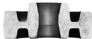
Flow structure of a hot-forged gear blank. Note how flow is parallel to all critical surfaces. (Courtesy of Bethlehem Steel Corporation, Bethlehem, PA.)
