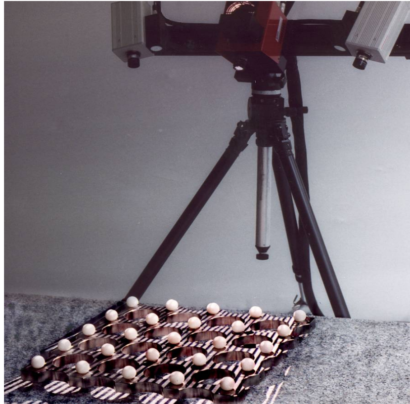
Optical 3D – Measurement in Volkswagen, ATOS (GOM). 77
