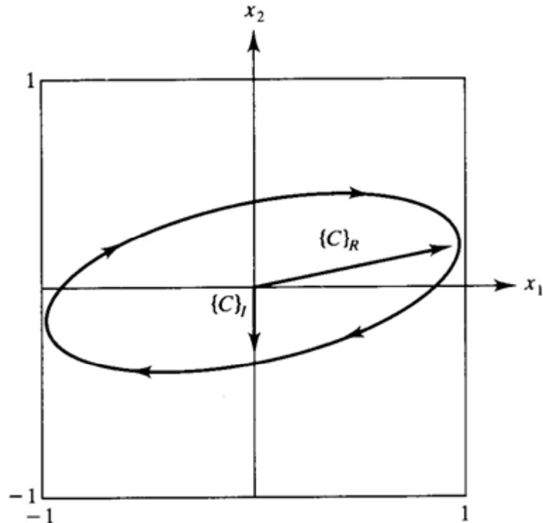
$$\mathbf{A} = \begin{bmatrix} -1 & 7 \\ -7 & -1 \end{bmatrix}, \quad \lambda_{1,2} = -1 \pm 7i, \quad \mathbf{c}_R = \begin{bmatrix} 1 \\ 0 \end{bmatrix}, \quad \mathbf{c}_I = \begin{bmatrix} 0 \\ 1 \end{bmatrix}$$
