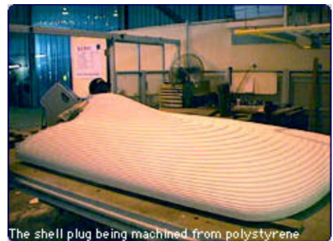
The shell plug being machined from polystyrene
