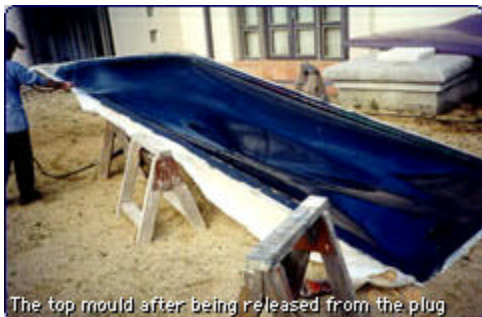
The top mould after being released from the plug
