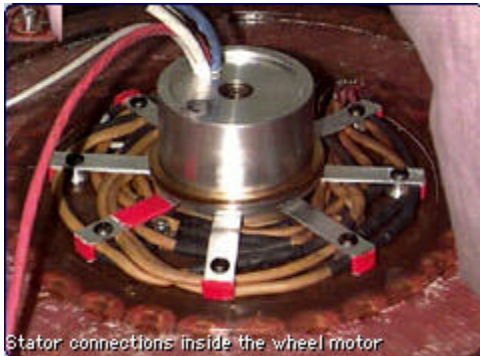
Stator connections inside the wheel motor
