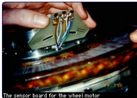
The sensor board for the wheel motor
