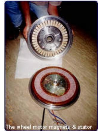
The wheel motor magnets & stator
