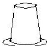
**"Automotive"** -- the round post familiar on starting batteries in gas-powered cars. The cable lug fits around the terminal.
