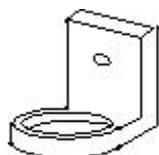
**"L"** -- A flat tang with a hole through it. A bolt through the hole connects the terminal to the cable lug.
