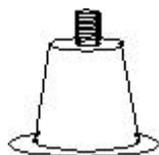
**"Universal"** -- Like an automotive post, with an extra stud in the center of the post. The cable lug fits over the stud and a nut holds them together
