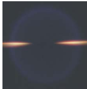
jet fuel burning in an oxygen/helium mixture (flame is blue and luminosity has disappeared)
